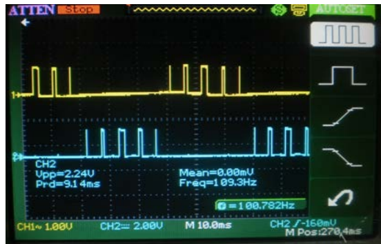
Figure 4. PWM pulse oscilloscope photograph of real measurements
