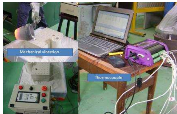
Fig. 4 The experimental set-up of composites casting
