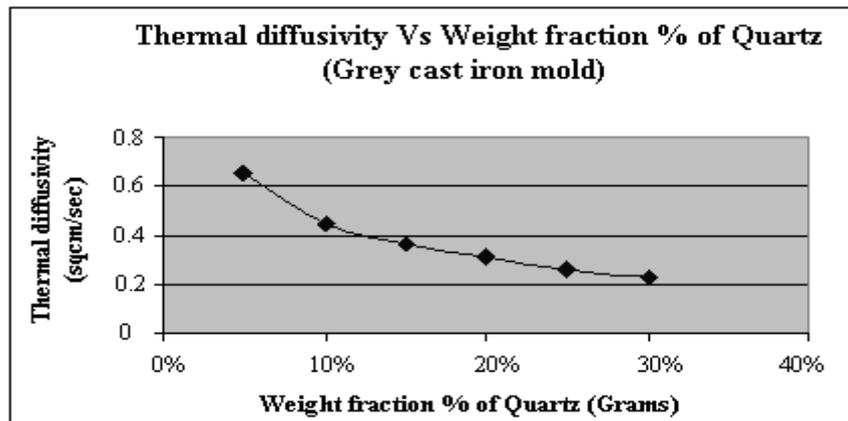
Figure 5 Thermal diffusivity Vs Wt Fraction % of quartz
