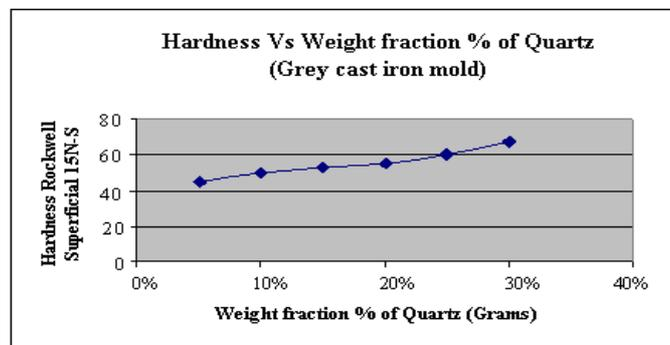
Fig. 3 Hardness Vs Wt Fraction % of quartz
