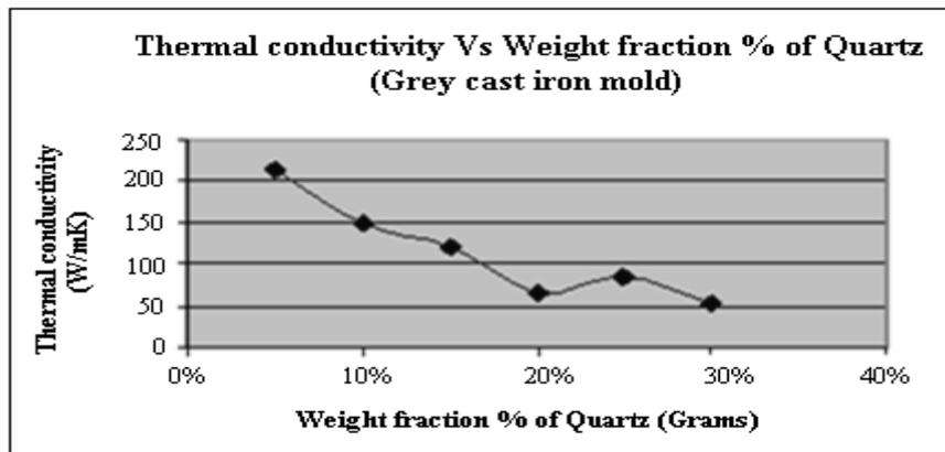
Figure 6 Thermal conductivity Vs Wt Fraction % of quartz
