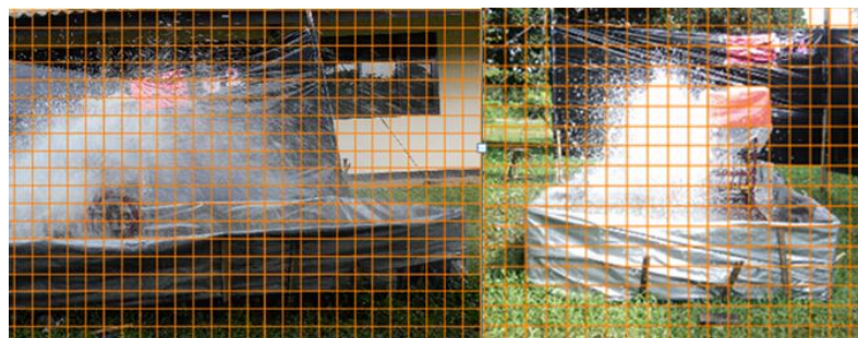
Figure 3. The image of water splash and calculation segment of splash coverage volume Torque occurred, electrical power consumption and splash coverage volume produced at different blade submerged shown in Table 1.
