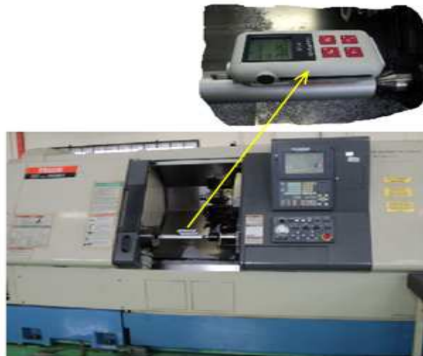
Fig. 4. Schematic view of measuring surface roughness
