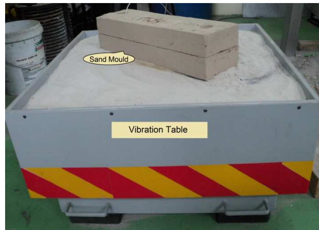
Fig. 2. Vibration table set up during solidification process of MMC
