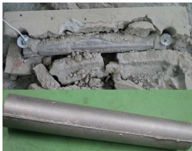
Fig. 3. The round bar casting product of MMC
