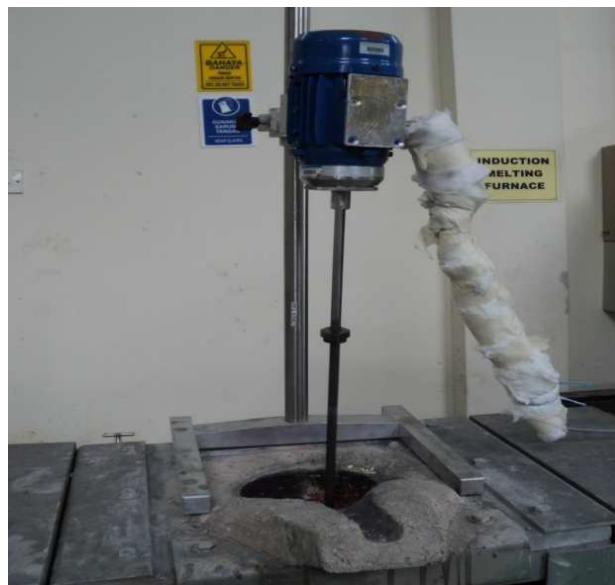
Fig. 1. Stirring process of liquid LM6 with the preheated TiC
