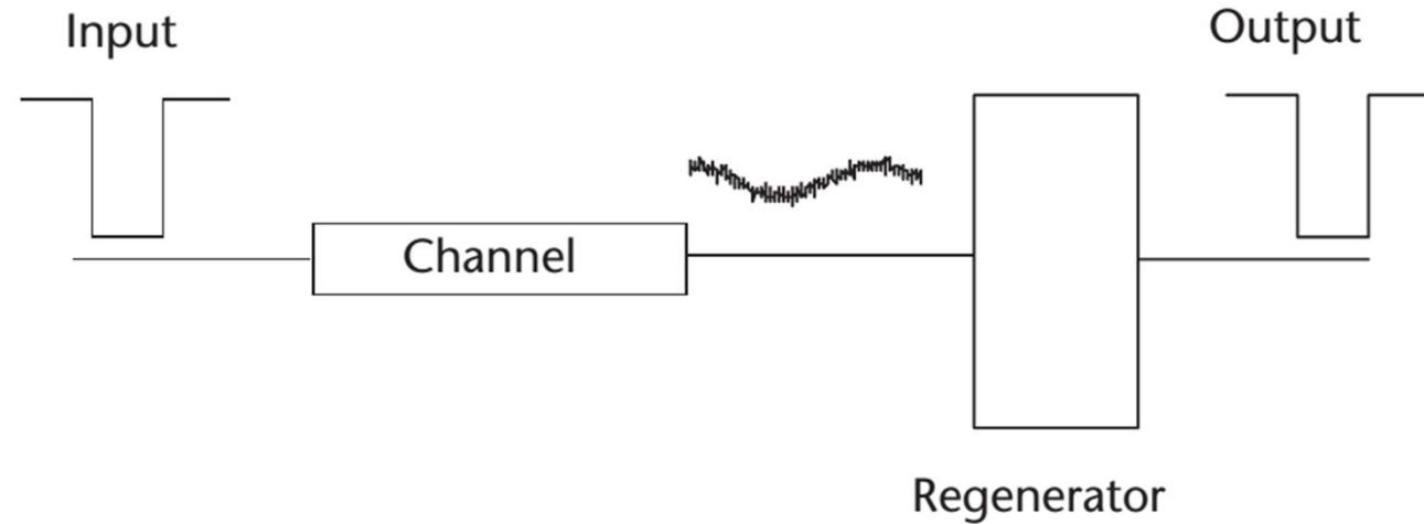
Amplifier (analog) versus Regenerator (digital)
