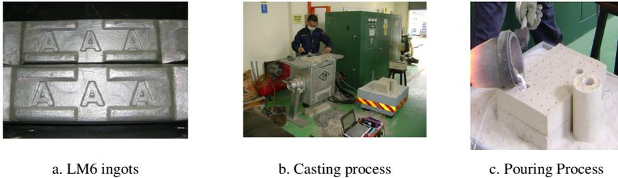
**FIGURE 1.** Processing of the composite specimen
