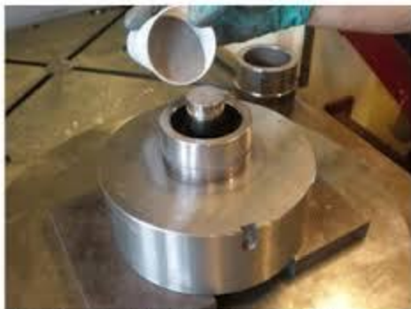
Fig. 2. Experimental tooling during powder fill (Courtesy Strecon)
