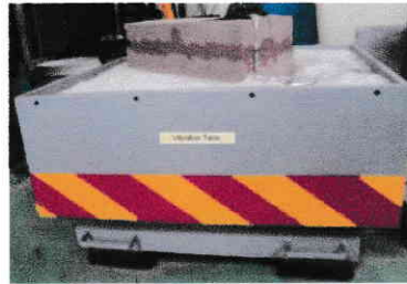
Figure 2. Vibration technique for solidification process
