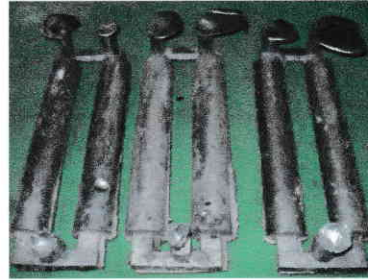
Figure 3. The round bar casting products of LM6 aluminum reinforced with 10 wt.% TiC particles.
