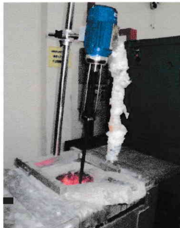
Figure 1. Stirring process of liquid LM6 with TiC particles
