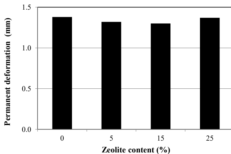
Fig. 4 Permanent deformation of tested SFP
