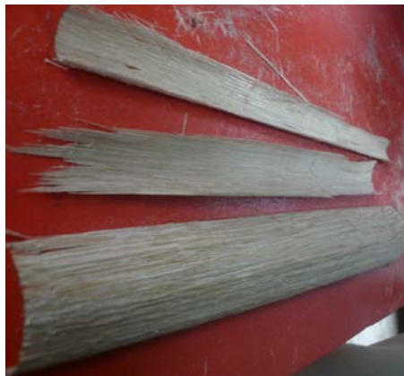
Figure 2. Veneerboo that was produced by the bamboo veneering machine Source: research team, 2009
