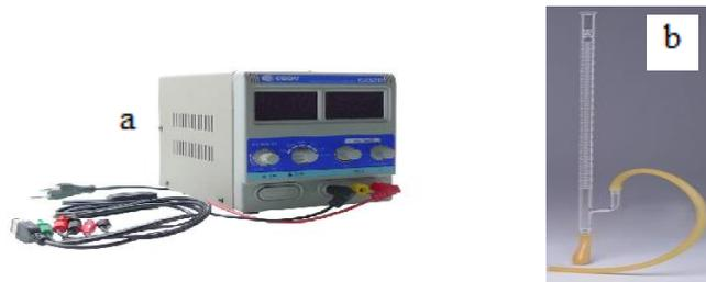
**Figure C.2:** Electrolysis devices, a) Power Supply, b) Bubble Flow meter
