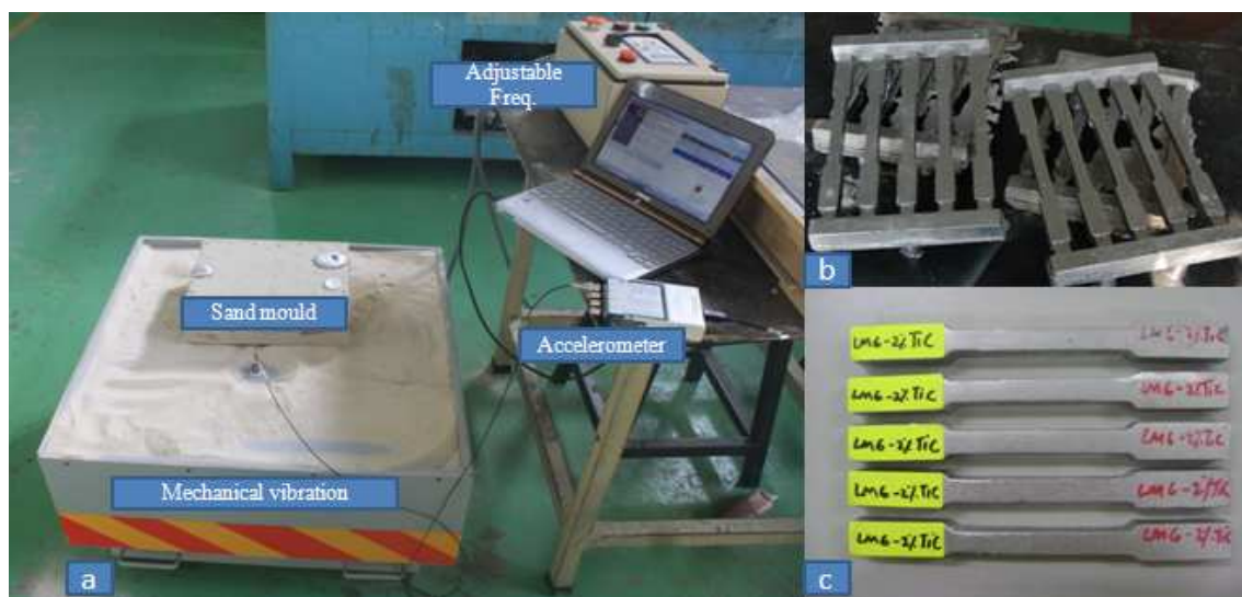
Figure 1 Vibration table setup (a), Specimens with the uncut gating system (b), Test specimens (c).
