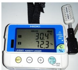
Gambar 6 Humidity logger HIOKI LR5001
