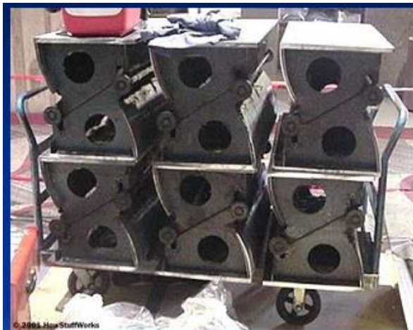
The individual steps from an escalator
