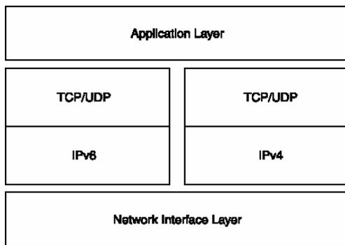
Fig1 Dual-Stack structure [7]
