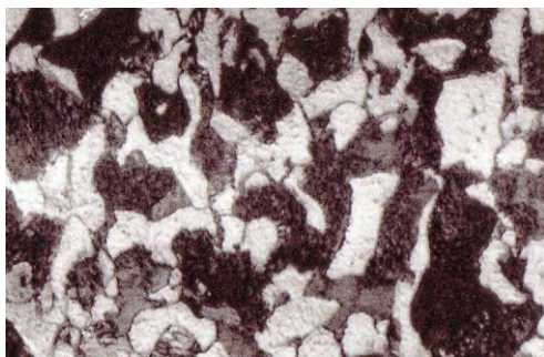
Fig. 3. The microstructure before hardening heat treatment. The ferrite (bright) and the pearlite (dark). 400x, 2%Nital
