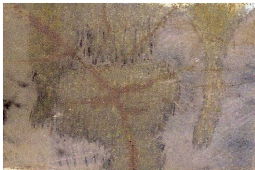
Fig. 9. The surface structure after hardening at 1000°C, holding time of 120 minutes. The crack appear due to cracking quenched
