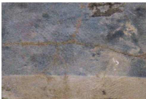
Fig. 5. The surface structure after hardening at 950°C, holding time of 60 minutes. The crack appear due to cracking quenched. 400X, 2%Nital
