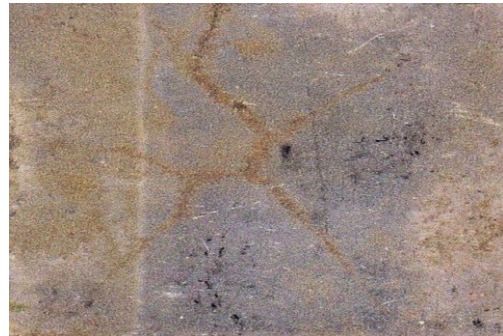
Fig. 8. The surface structure after hardening at 1000°C, holding time of 60 minutes. The crack appear due to cracking quenched. 400X, 2%Nital
