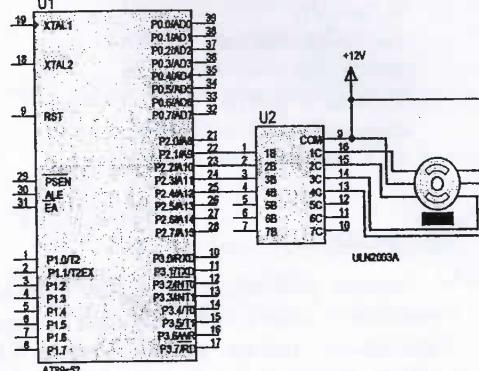
Gambar 5. Driver Motor Stepper
