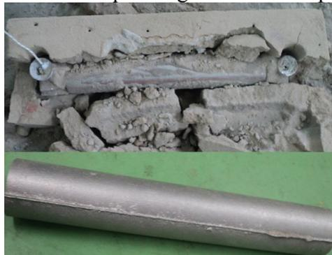
Fig. 3. The round bar casting product of TiC reinforced LM6 aluminium composite
