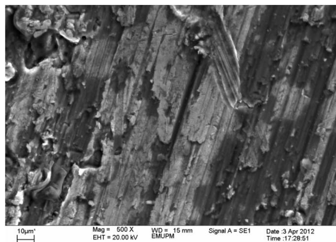
Fig. 4. The microstructure of LM6 aluminium alloy reinforced 10 wt.%TiC composite
