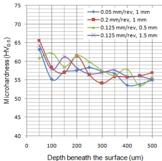
Fig. 7. The microhardness when machining of LM6-TiC composite at cutting speed of 250 m min<sup>-1</sup>
