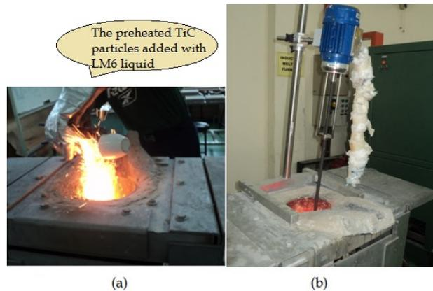
Fig.1. (a) Mixing process of preheated TiC particle with LM6 liquid
