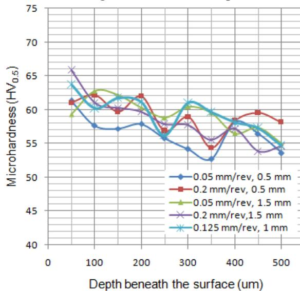
Fig. 6. The microhardness when machining of LM6-TiC composite at cutting speed of 175 m min<sup>-1</sup>
