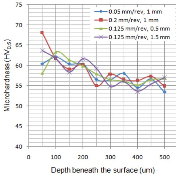
Fig. 5. The microhardness when machining of LM6-TiC composite at cutting speed of 100 m min<sup>-1</sup>
