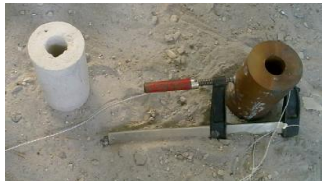
Figure 1 Sand and permanent metallic mould
