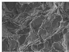
b. Fractograph of 0.2% TiC at 300X magnification
