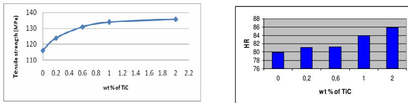
a. Average tensile test versus weight fraction of TiC
