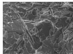
c. Fractograph of 0.6% TiC at 300X magnification
