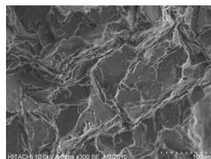
a. Fractograph of LM6 at 300X magnification
