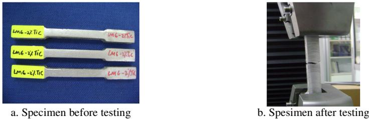
**FIGURE 2.** Tensile Speciment of composite
