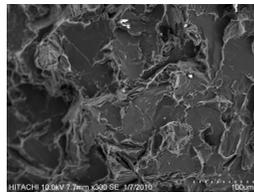
d. Fractograph of 1% TiC at 300X magnification
