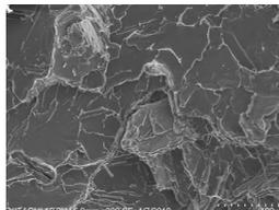
e. Fractograph of 2% TiC at 300X magnification
